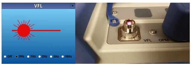
Pictured: Visual Fault Locator (VFL) beam illuminates bends, splices, and faults in optical fibers, with an effective range of up to 10km.
